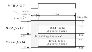
Figure 7-22: Active video for ITU-R BT.601, NTSC
