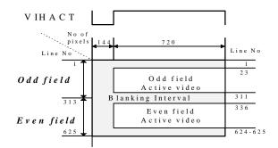
Figure 7-23: Active video for ITU-R BT.601, PAL
