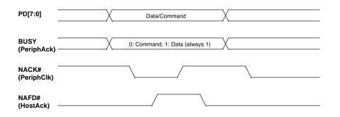
Figure 7-12: ECP Reverse Timing
