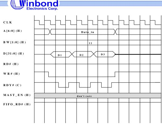
Figure 7-17: Write cycles to Vdata\_in register, BW[1:0]=11
