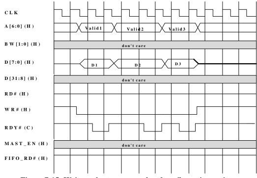
Figure 7-15: Write cycles to command and configuration registers
