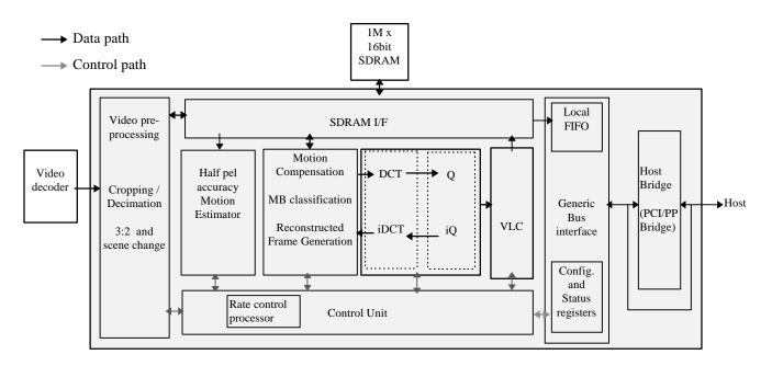
Figure 6-1: W99200F block diagram
