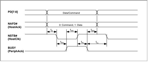
**Figure 9-7: ECP Forward Timing**
