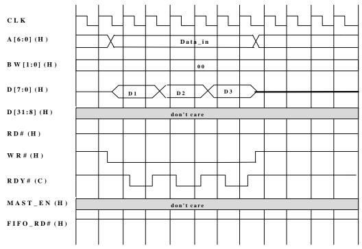
Figure 7-16: Write cycles to Vdata\_in register, BW[1:0]=00
