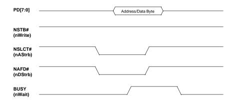
Figure 7-9: EPP Data or Address Read Timing
