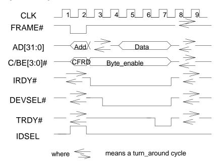
Figure 7-2: PCI Configuration Read Timing
