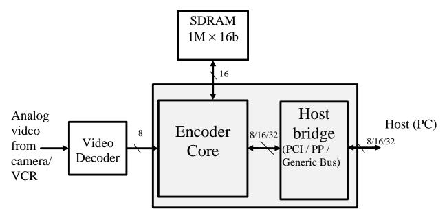
Figure 1-1: A video encoding system based on the W99200F chip
