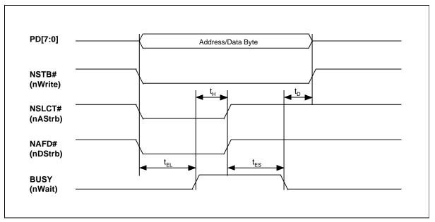
Figure 9-6: EPP Data or Address Write Timing
