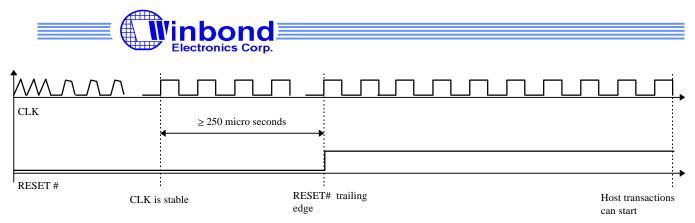
Figure 7-28: CLK and RESET# after power up
