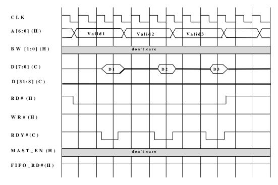
Figure 7-14: Read cycles from configuration and status registers
