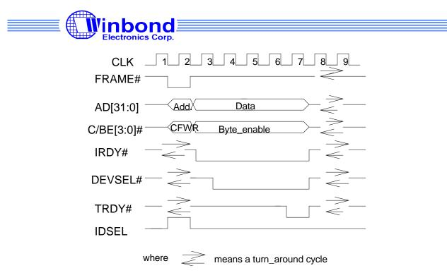
Figure 7-3: PCI Configuration Write Timing
