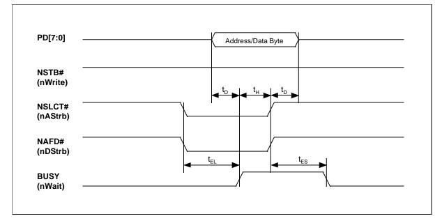
Figure 9-5: EPP Data or Address Read Timing
