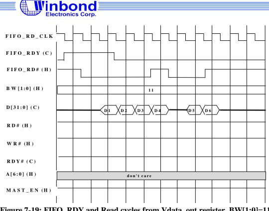
Figure 7-19: FIFO\_RDY and Read cycles from Vdata\_out register, BW[1:0]=11
